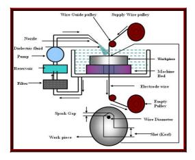
Fig. 8 wire cut EDM
