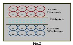
**B.** *Breakdown*-Dielectric breakdown, creation of the plasma channel
