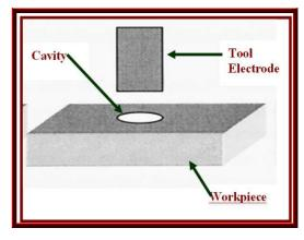
Fig.7 Die Sinking EDM
