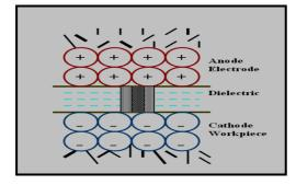
Fig.4 **D. End of the discharge**: plasma implosion, removing of the molten metal pool.
