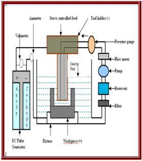
Fig. 1 Schematic of EDM Process
