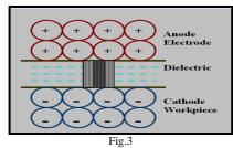
C. *Discharge*-Heating, melting and vaporizing of the workpiece material
