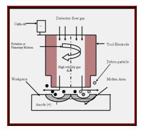
Fig. 9 Principle of Dry EDM
