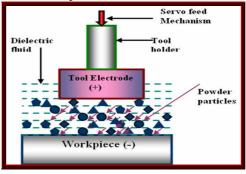
Fig.10 working principle of PMEDM
